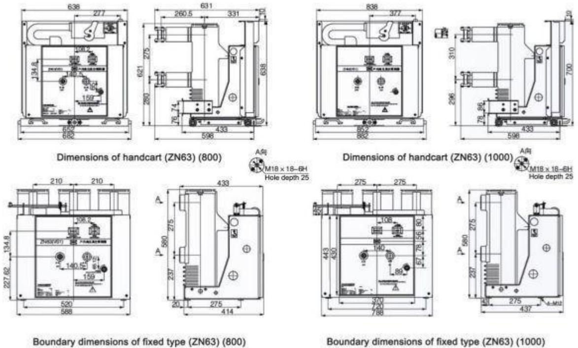
**Timetric Indoor Solid Sealed Vacuum Circuit Breaker Parameter (Specification)**
